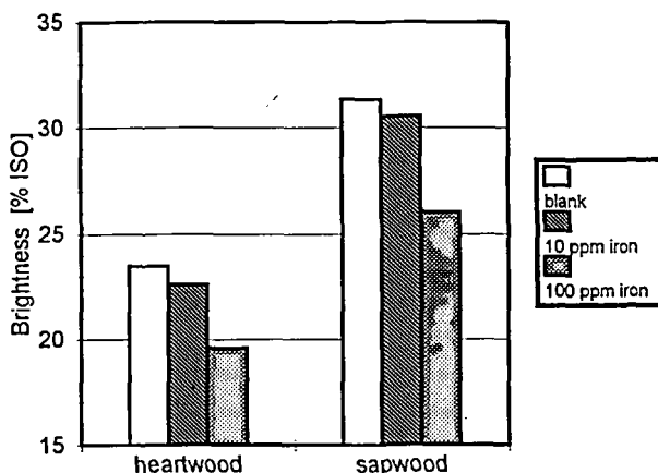
FIGURE 2. Effect of iron (III) (in \mu\text{g/g} wood meal) on the brightness of Douglas fir wood meal. Samples were heated to 135^\circ\text{C} for 5 min.
